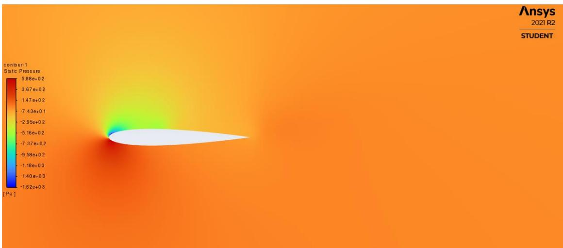
**Figure 16.** Pressure contour at 10 degrees AoA
