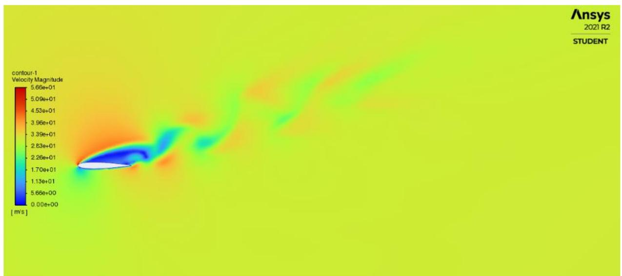
**Figure 13.** Velocity contour at 20 degrees AoA
